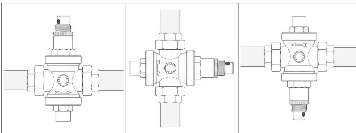
Please check that the flow direction is concurrent to the arrow on the reducer body. Commissioning and pressure set-up is done by rotating the brass spring holder on the top; to do it (see pictures below), loosen the plastic lock ring, turn the spring holder using a screwdriver (clockwise to increase outlet pressure, counter clockwise to decrease outlet pressure), tighten the plastic ring.
